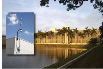
"Built to withstand all kinds of weather, the state-of-the-art WeatherBug Tracking Station (inset) is currently installed atop a building located at MDC's North Campus, where it records 27 different real-time weather measurements. Live weather data is available now online at http://weather.weatherbug.com/ . The online weather network provides live local weather conditions, forecasts, and severe weather alerts."
